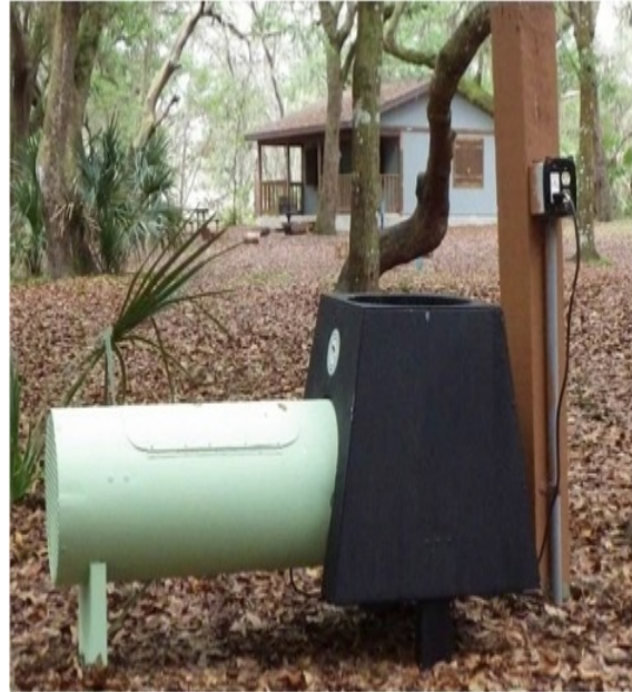
Pasco suction trap, originally called “mini-bidlies” because they are a mini version of the Bidlingmayer trap that was developed at FMEL.
