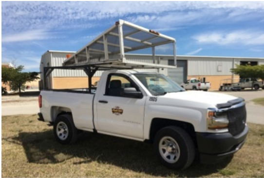
Bidlingmayer truck trap used to sample airborne mosquitoes.
