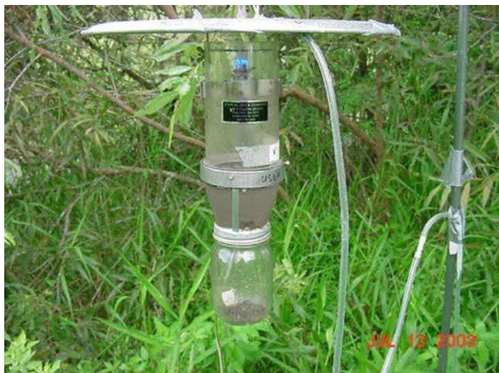
Experimental light emitting diode CDC light trap using blue light to attract mosquitoes. Colored light LEDs use little power compared to incandescent lamps and are highly attractive to certain mosquito species.
